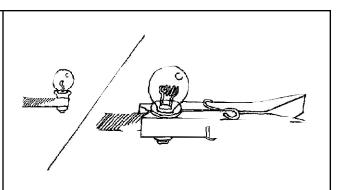
2. Fold the short foil strip in half lengthwise, so it's thinner. Wrap one end around the bulb and pinch the bulb in the clothespin.
