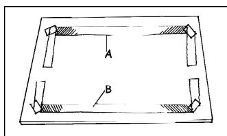
Set one of the long strips of foil along one long edge of the cardboard, fold up the ends, and tape them in place. (See " A," above). Then fold and tape the other long strip down on the other long edge.
