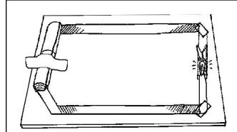
5. The two loose ends of the foil strips make up the switch. Touch the ends together to complete the circuit. What happens?
