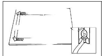
**3.** Set the clothespin, with the bulb in it, on top of the end of the top foil strip. Make sure the bottom of the bulb touches the foil strip. Tape it in place.
